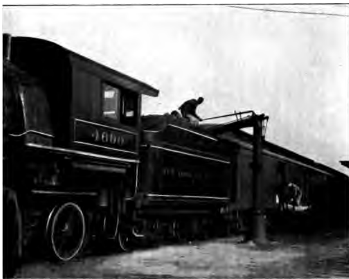
WHEN THE TRAIN COMES TO A WATER STATION THE FIREMAN GETS OUT AND FILLS THE TANK "
